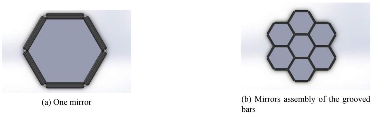
Fig. 2-9 Model of the grooved bars assembly
