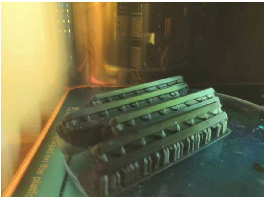
Fig. 2-7 3D printing of the bars with resin
